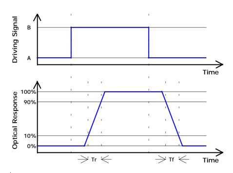
Level A - Level B  $\geq$  16 then  $T_r \leq$  16 ms &  $T_f \leq$  16 ms
